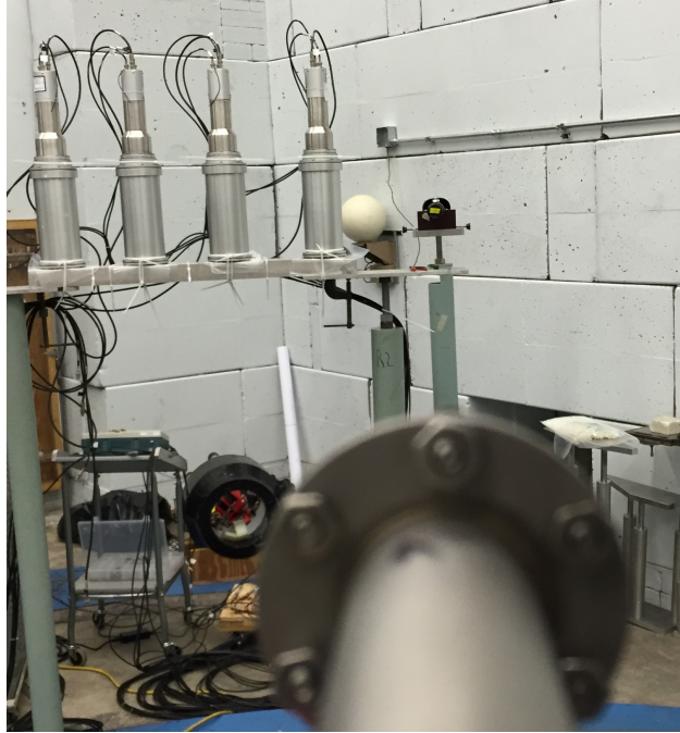
Figure 7.7: Photograph taken looking along the proton beam direction just upstream of the neutron production target, which is obscured from view and held in place behind the visible flange in the bottom right of the image. The 4 large detectors visible in the middle-left of the image are the custom EJ-301 cells from Eljen. Quasi-monoenergetic neutron beams were produced using the {}^7\text{Li}(p,n) reaction; several different proton energies were used to produce neutron beams of different energies. As each detector was located at a slightly different neutron-emission angle with respect to the production target, each detector was subject to slightly different beam energies. From Reference [211].
