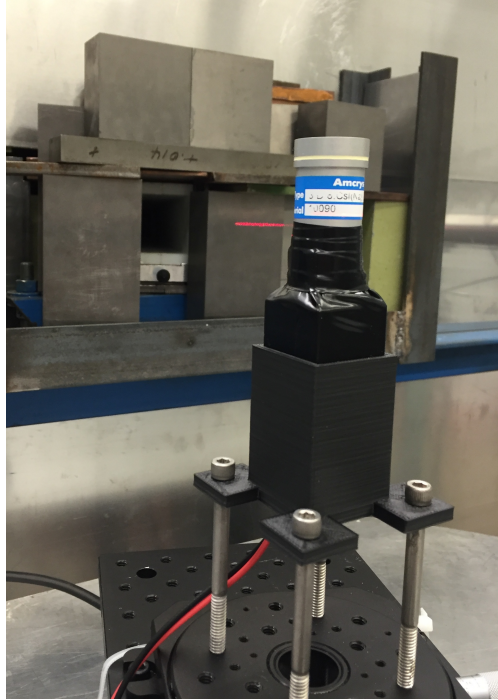
Figure 4.7: Photograph of the CsI[Na] detector assembly and its associated PMT mounted for the QF measurement at the SSA. Comparison of the realized assembly and its concept design, shown in Figure 4.6, shows some deviation from the original design. The end of the SSA neutron-beam collimator is visible in the background.
